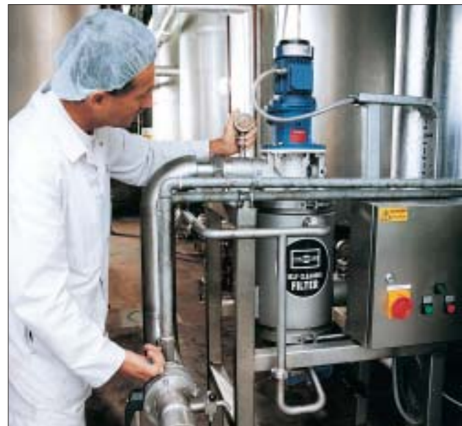
Russell Eco Self-Cleaning Filters® aid quality control procedures for filtering liquid chocolate at Walls Ice Cream.
