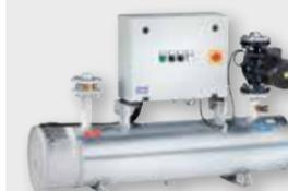
The KVE units are used to keep the temperature of cooling water circuits in large diesel engines at operating value. This means the engines remain ready to start at any time. The KVE series is available with heating power from 3 to 600 kW. The circulation pump and power unit are integrated and perfectly adapted for the application.
