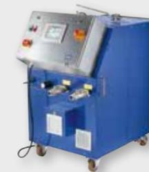
Compact & mobile system for preheating gearboxes and engines on the test rig and on the racing track. Additional functions: flushing test rigs with clean oil, evacuating the external system with compressed air. With adjustable pump power and heated tank with level monitoring. Operation via touch display.
